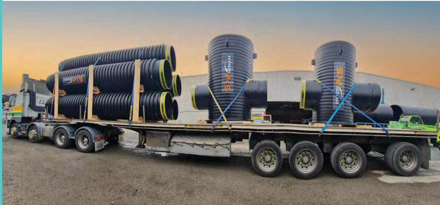
Post-consumer plastic is getting a second life at Hynds PKS in Christchurch. The site is the sole manufacturer of Supaduct™ Rural, a lightweight and durable culvert pipe system produced from reprocessed raw HDPE (high density polyethylene) material and post-consumer recycled plastic.
